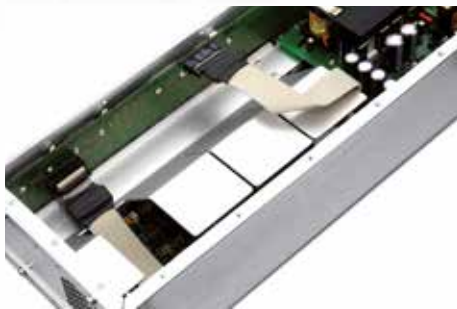
Heat conduction plate, aluminium
