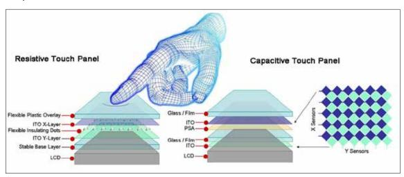
Resistive touchscreens react to pressure, which connects two electrically conductive layers at a specific point. This technology ensures easy operation using fingers, gloved fingers and pens. The surface is relatively resistant to dirt and is usually made of plastic.
