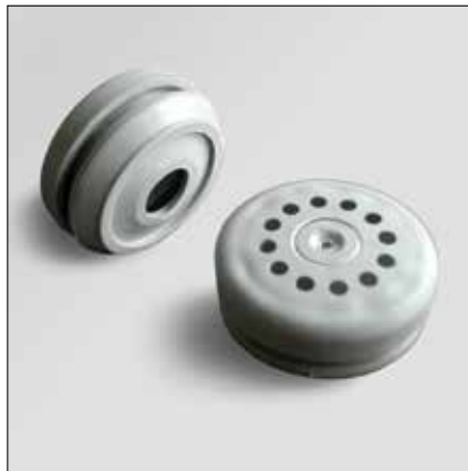
Ventilation plug with labyrinth seal to prevent the formation of condensation; IP x 4; for wall thicknesses of 1.5 - 4.5 mm
